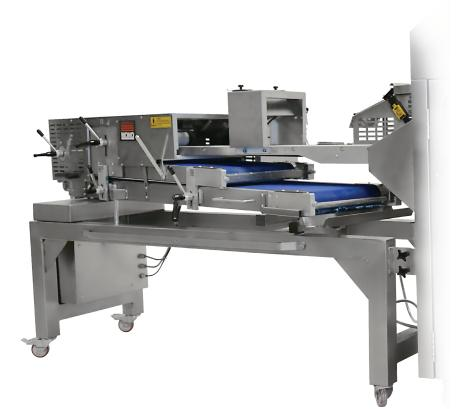
Roll Forming Unit can produce a variety of products including a selection of flattened hamburger rolls, petit pain and elongated hotdog/finger rolls.
